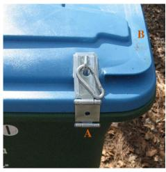
3. Lay the hinge over the lid to mark the best position for the eye of the hasp. Make sure the hinge can be locked and unlocked easily. Pre-drill  $\frac{3}{16}$  holes in the marked spots on the lid of the can for the hasp eye.
